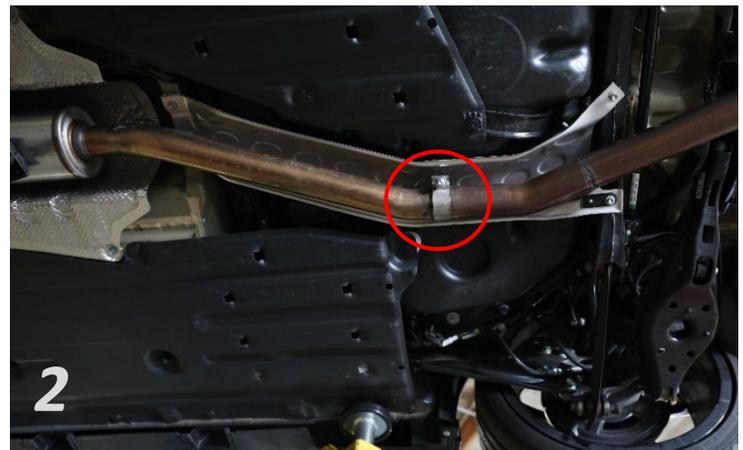
1. **(Read instructions prior to installation.)** It is recommended to not fully tighten the exhaust until it has been fully installed. Leave loose for adjustability.
