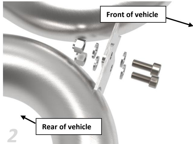
1. **(Read instructions prior to installation.)** It is recommended to not fully tighten the exhaust until it has been fully installed. Leave loose for adjustability.
