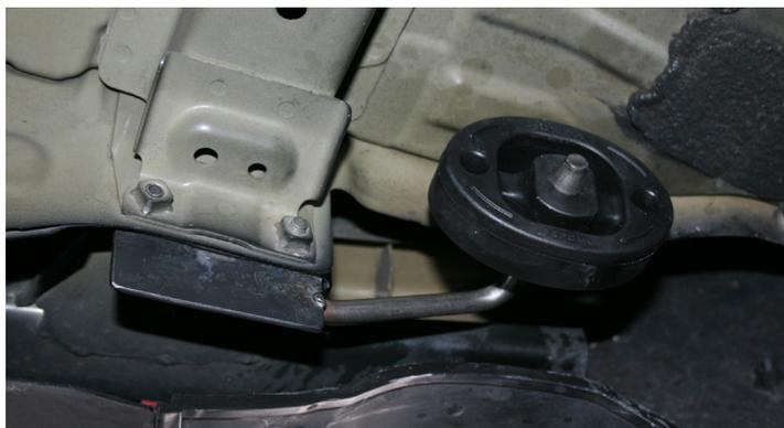
**Step 8:** Install the resonator pipe rubber hanger mount back onto the chassis and the original (x3) nuts removed from step 3 and tighten.
