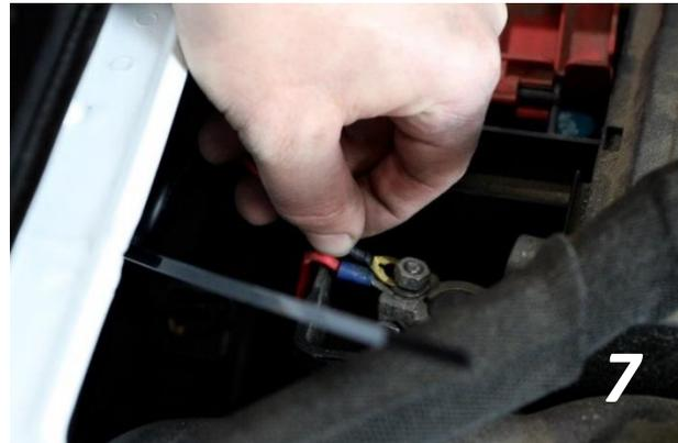
18. Connect the wire harness together and tuck the remaining wire into the frame. Organize any other loose wires and secure with remaining zip ties.
