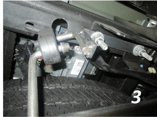
11. Next Install the Over-Axle, but do not fully tighten the band clamp.
