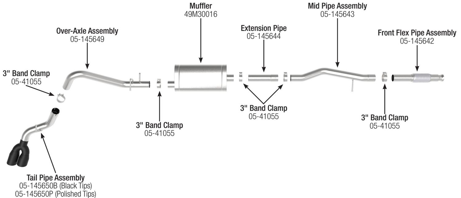
**Caution:** aFe recommends professional installation on our products. Allow time for your vehicle to cool down prior to installation. When working on or under your vehicle proceed with caution. Exhaust systems reach high temperatures and may cause serious burns. Wear protective safety equipment; eye goggles and gloves to ensure a safe installation.
