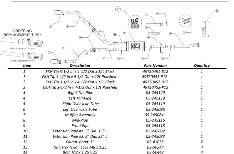
**aFe POWER recommends professional installation on this product.** Thoroughly inspect the aFe POWER exhaust system to make sure there is no damage from shipping (if damage is noted, immediately contact aFe POWER customer service). Allow time for your vehicle to cool down prior to installation. When working on your vehicle proceed with caution. Wear protective safety equipment; eye goggles and gloves to ensure a safe installation.
