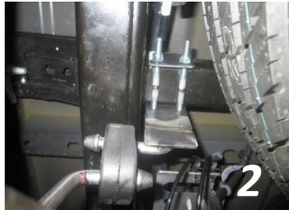
11. Install the left driver side tail-pipe, but do not fully tighten.
