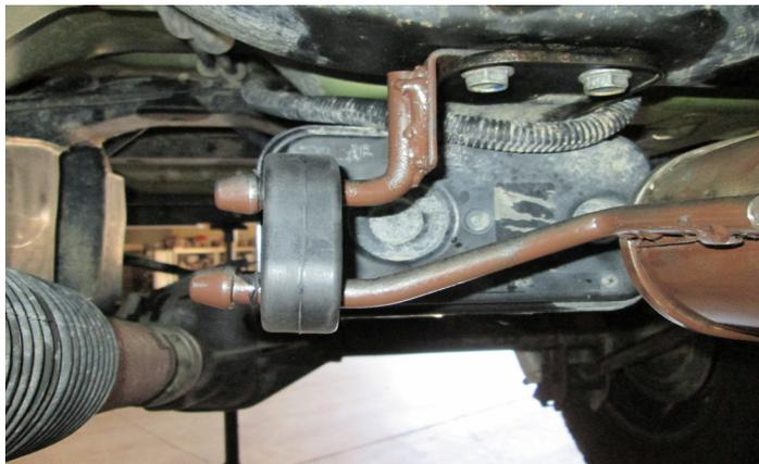
**Step 10:** Using (x1) supplied 2.5" band clamp, install the aFe Tail Pipe onto the Muffler Pipe and rubber hanger mounts but do not tighten.
