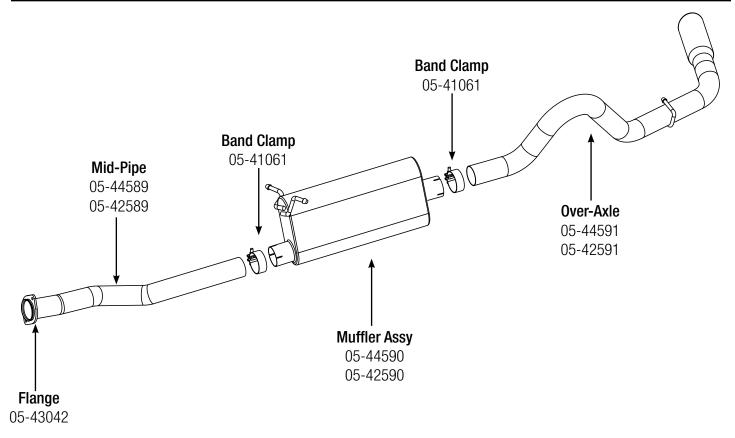
**Step 1: (Read Instructions prior to installation)** Remove your stock exhaust from the rear of your truck working your way forward. Take caution not to damage the factory isolation mounts as they will be reused. It may be helpful to lubricate the isolation mounts prior to disassembly. It is recommended to not fully tighten the clamps until the entire system has been installed.
