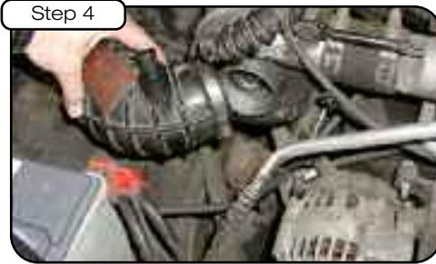
Remove factory rubber elbow at turbo.
