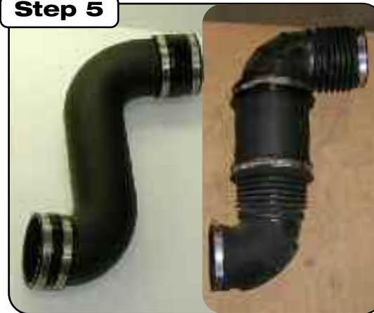
Compare the difference between stock and the Torque Booster Tube. Re-check clamps and connections and retighten after a few hours of operation.
