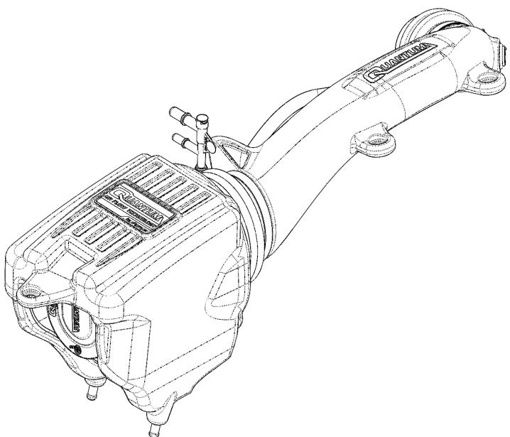
advanced FLOW engineering Quantum Cold Air Intake System
