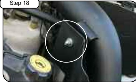
Install flat/wavy washers and nut to isolation mount. Tighten both sides with 10mm socket or wrench.
