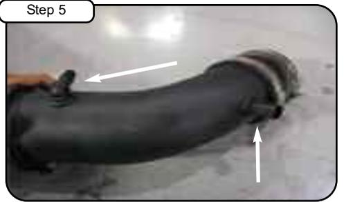
Step 5 Install air temp sensor and 1/2" fitting into new tube with grommet(s) provided. Place hump coupler with clamps provided onto tube.
