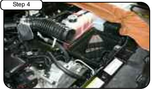
Step 4 Loosen and remove OE intake tube with 5/16" nut driver. Remove bottom air box out of vehicle. Remove air temp sensor.
