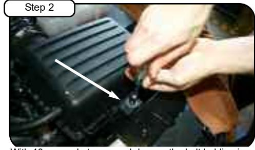
Step 2 With 10mm socket or wrench loosen the bolt holding in upper half of OE air box. (Save for step 8)
