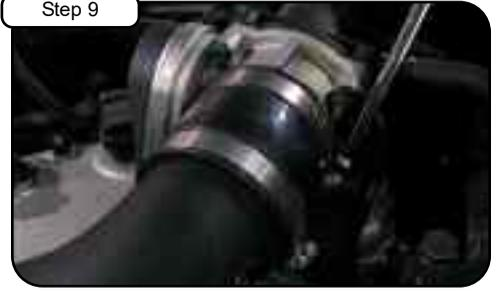
Step 9 Tighten clamps using 5/16" nut driver.
