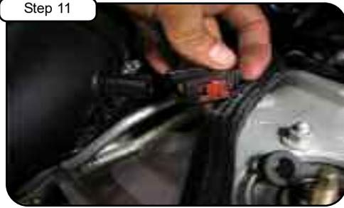
Step 11 Re-connect air temp sensor harness.
