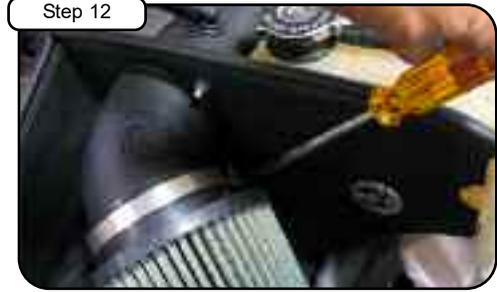
Step 12 Install air filter and tighten using 5/16" nut driver.
