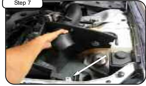
Step 7 Install intake into vehicle. Position housing to tab.
