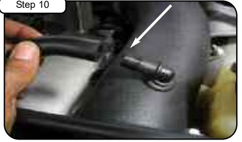
Step 10 Re-connect crank case line to fitting on tube.
