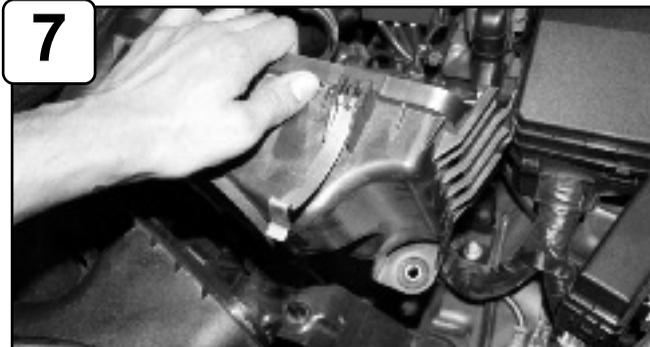
Lift and remove bottom half of air box out of vehicle.
