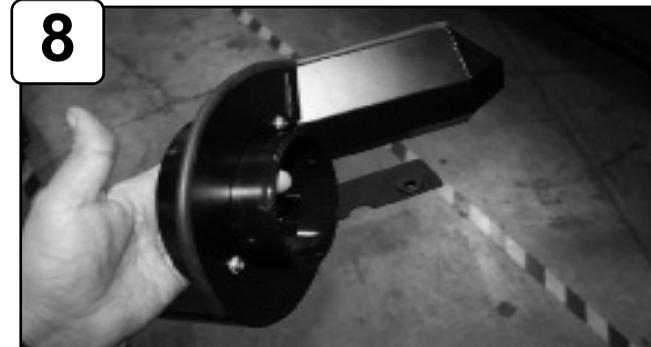
Install filter adaptor to housing and secure using button head screws provided. Tighten using 4mm allen key. Attach rubber trim to top of housing.
