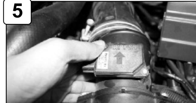
Pull back MAF sensor from intake tube.
