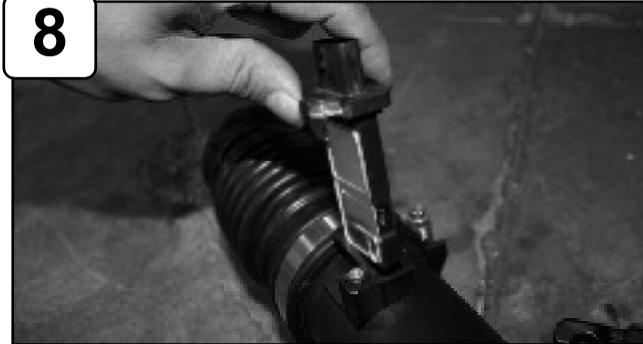
Remove MAF sensor from stock intake.
