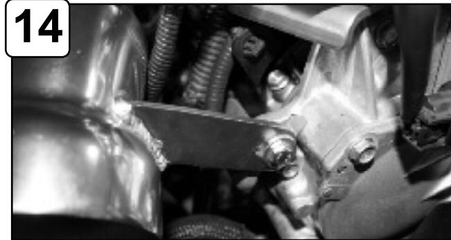
**14** Secure tab to engine and tighten using provided M6 screw and flat washer.
