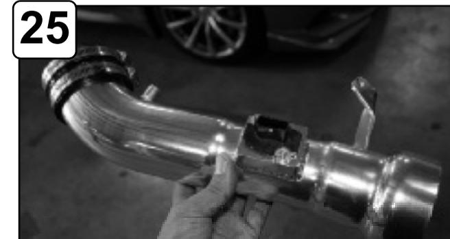
25 Attach coupling with clamps to tube.
