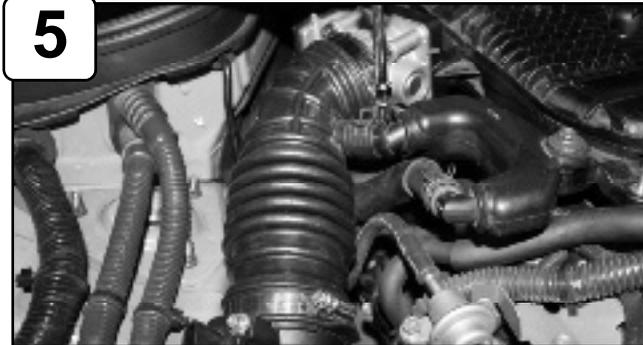
Loosen clamps on intake using 5/16" nut driver.
