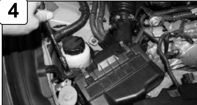
Disconnect MAF sensor harness. With 10mm socket or wrench loosen bolt holding in air box.
