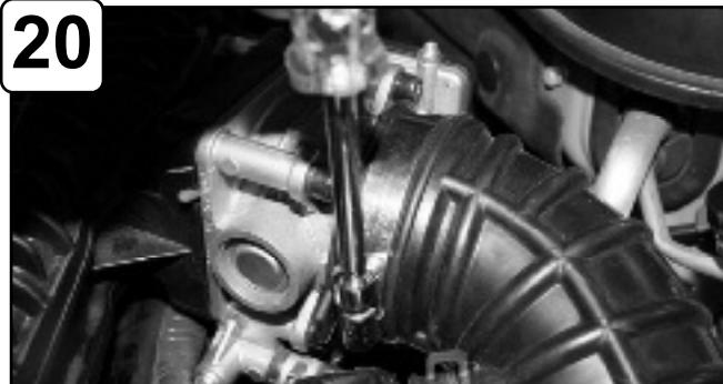
20 Disconnect MAF sensor harness. Loosen clamps using 5/16" nut driver.
