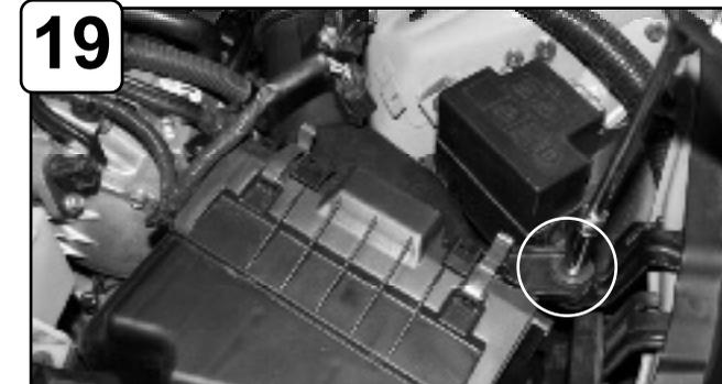
19 With 10mm socket or wrench, loosen the bolt holding in air box.
