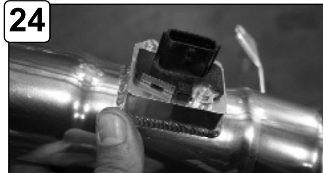
24 Install MAF sensor to new tube using provided M4 screws.
