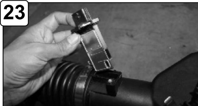
23 Remove MAF sensor from stock intake.
