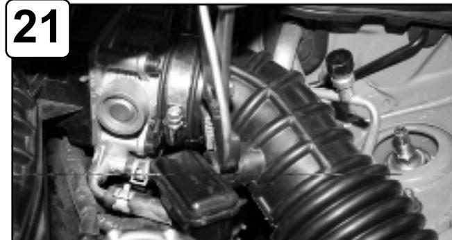
21 With pliers pull back stock intake tube from vent box.
