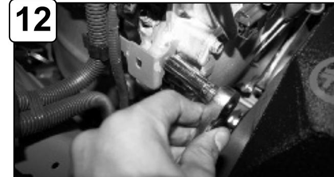
**12** Loosen bolt on engine securing harness bracket.
