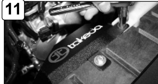
**11** Install housing and secure to radiator support and tighten using bolt from previous step. Secure other tab using provided M6 screw, flat washers and nut.
