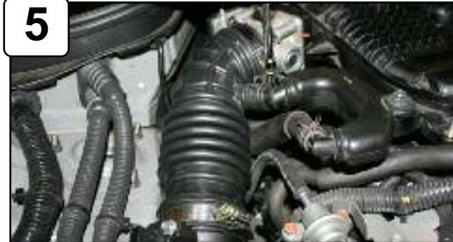
Loosen clamps on intake using 5/16" nut driver.
