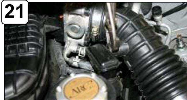
Disconnect the crank case line using pliers.
