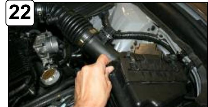
Remove complete intake out of vehicle.
