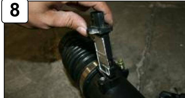
Remove MAF sensor from stock intake.
