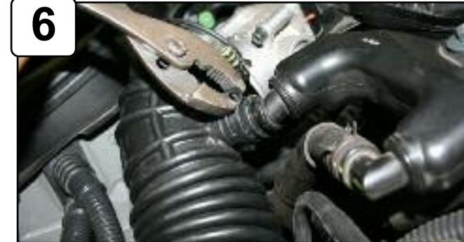
Disconnect the crank case line from the intake tube using pliers.
