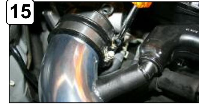
15 Tighten all clamps using 5/16" nut driver. Attach the crank case line using the provided 5/8" hose.
