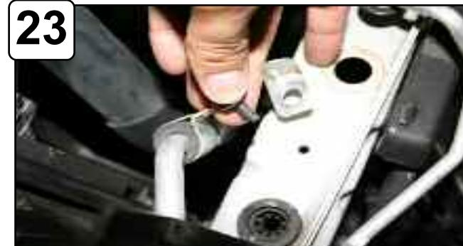
23 Loosen bolt holding in radiator fan & A/C bracket with 10mm socket or wrench. (To be used in step 24A) Loosen bolt holding in radiator fan bracket with 10mm socket or wrench. (To be used in step 24C.)
