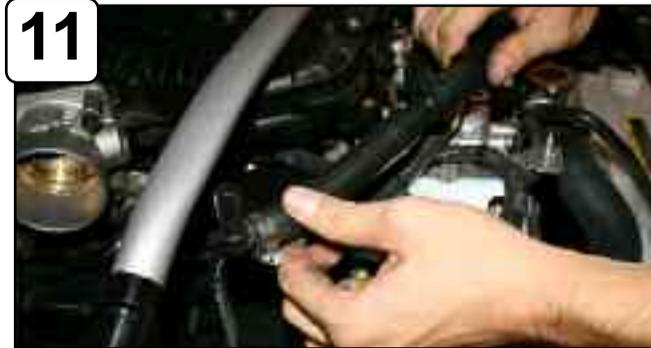
With 6" L 5/8" hose, 1/2" plastic elbow and mini clamp provided tighten at end of hose. On other end with 5/8" straight fitting, connect to stock crankcase line. Make sure 1/2" elbow is facing up under intake tube side. see step 14
