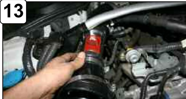
Install into vehicle and position tube. (Elbow coupler on throttle body and reducer coupler on filter adaptor) Do not tighten clamps.
