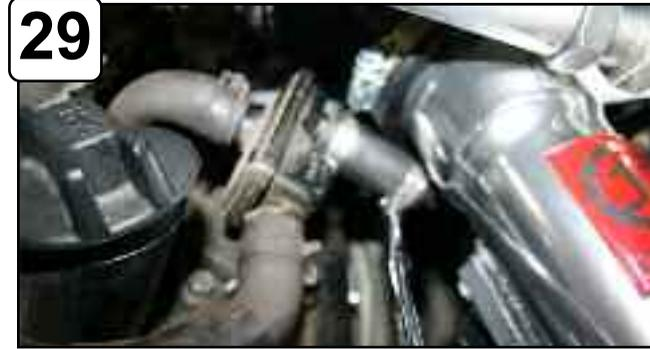
From step 26, install 1/2" plastic fitting into rubber grommet on bottom of tube. *Make sure fitting is inside of tube.*
