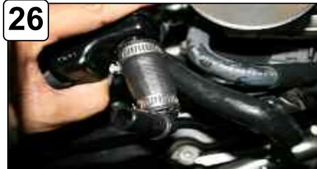
26 With 3"L 5/8" hose, 1/2" plastic elbow & mini clamps provided tighten at end of hose. Attach other end of hose to vent box with mini clamp and tighten. Make sure 1/2" elbow is facing up under intake tube side. see step 29
