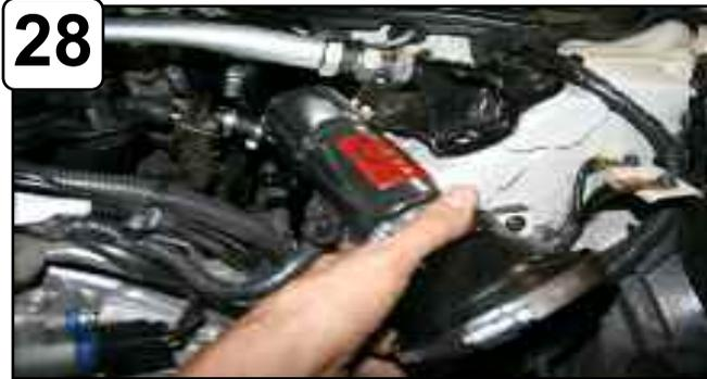
Install into vehicle and position tube. (Elbow coupler on throttle body and reducer coupler on filter adaptor)
