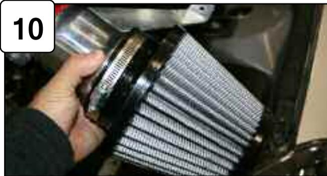
Attach air filter to intake tube and tighten clamp using 5/16" nut driver.
