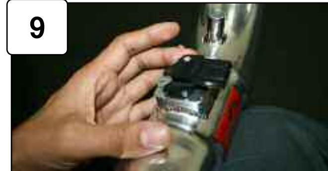
Remove MAF sensor from stock intake. Install into new intake tube and secure using provided M4 screws.
