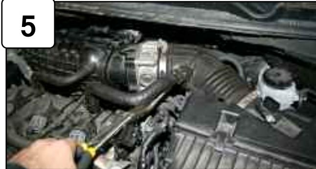
Remove crank case line from intake tube using pliers.
