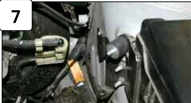
Install M6 male/female isolation mount to ECU harness bracket and secure.
