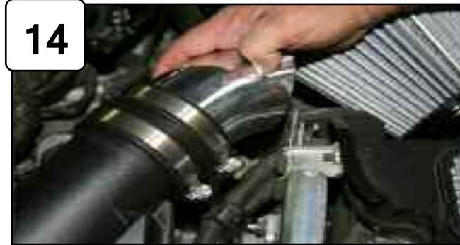
Install cold air duct using coupler with clamps provided. Using screw, nut and washer provided, tighten tab on duct to bracket using 10mm socket or wrench. Tighten clamps using 5/16" nut driver.
