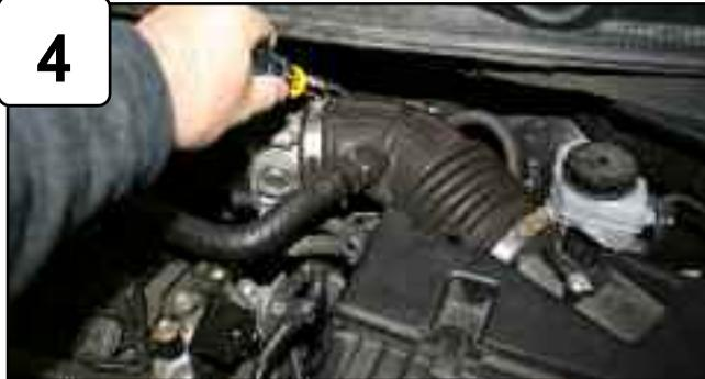
Disconnect MAF sensor harness. Loosen clamp on throttle body.
