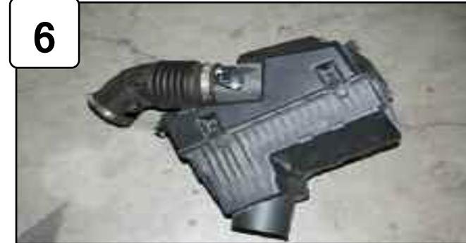
Remove stock intake out of vehicle.
