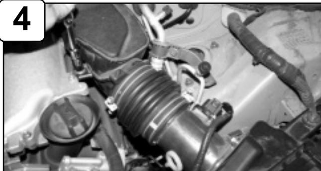
With 10mm socket and ratchet, remove the two 10mm bolts from the OEM intake tube and airbox. Loosen the top of OEM intake tube w/ 5/16" nut driver.
