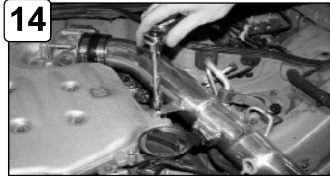
**14** Secure tube and tighten using M6 screw and washer provided. Tighten using 10mm socket or wrench.
