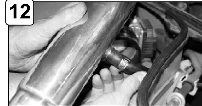
**12** Attach crank case line to intake tube.
