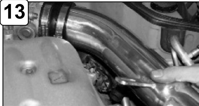
**13** Insert tube into couplings. Locate hole on tab to mounting location on engine plenum.
