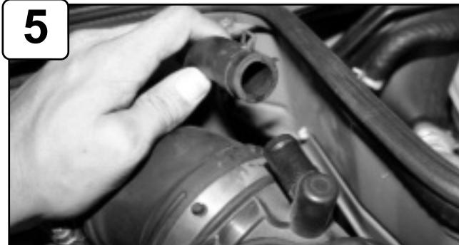
Remove crank case line from stock intake tube. Disconnect MAF sensor harness.
