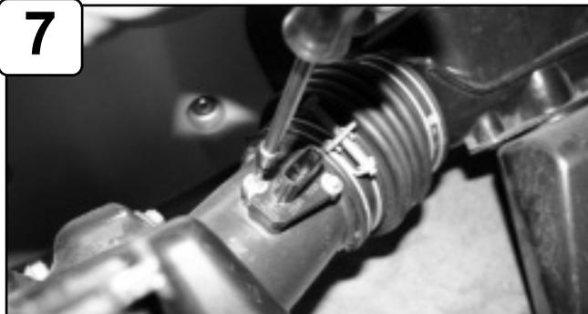
With T20 Torx bit, loosen the 2 bolts holding in MAF sensor. Carefully remove sensor out of stock intake.
