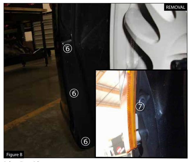
Refer to Figure B for step 6 Step 6: Remove the three push clips on the driver side inside fender well 6 connecting to the bumper, and also the one by the amber light 7.
