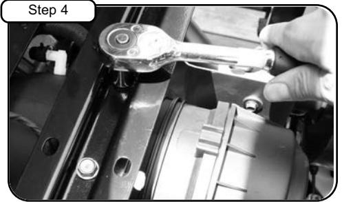
Loosen two bolts on intake housing.
