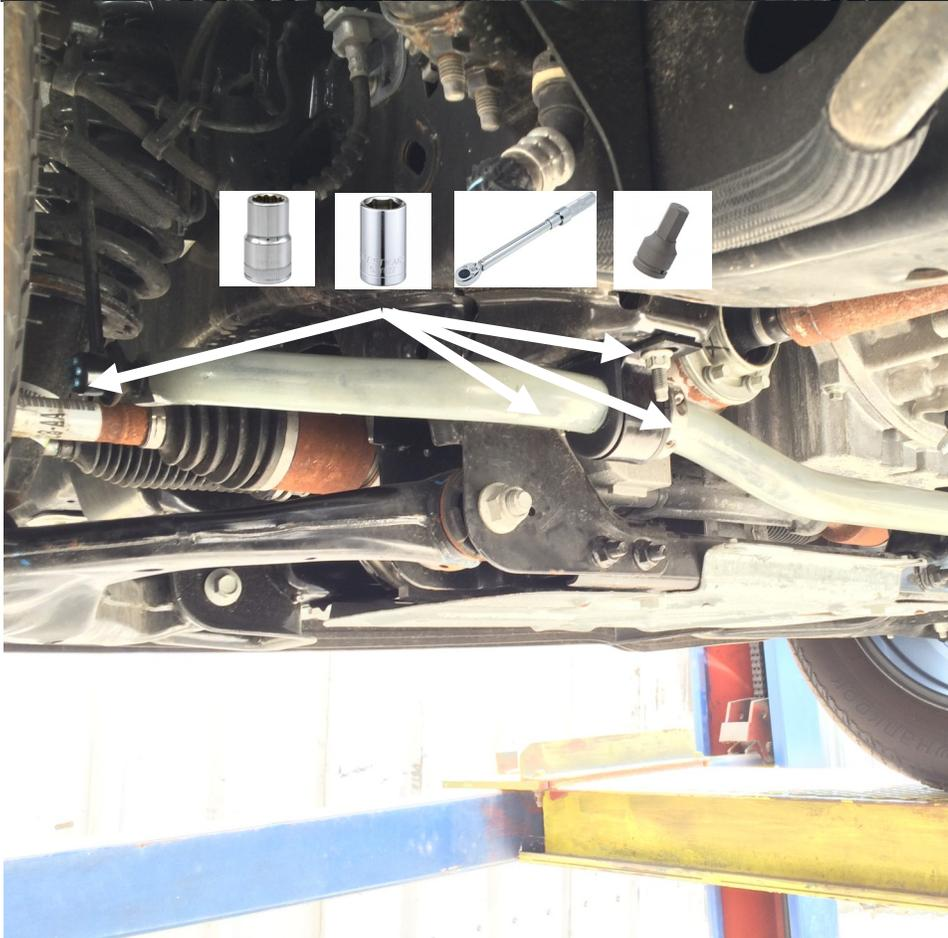
Revisit each of the fasteners and torque to the specified torque table below.
