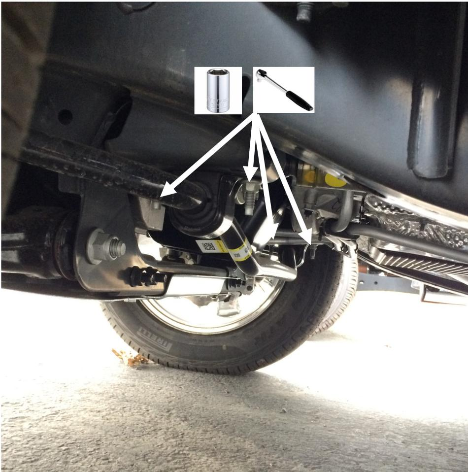
With the end-links free from the sway bar. Remove the 4 nuts holding the sway bar in place with a 15mm deep socket and ratchet.
