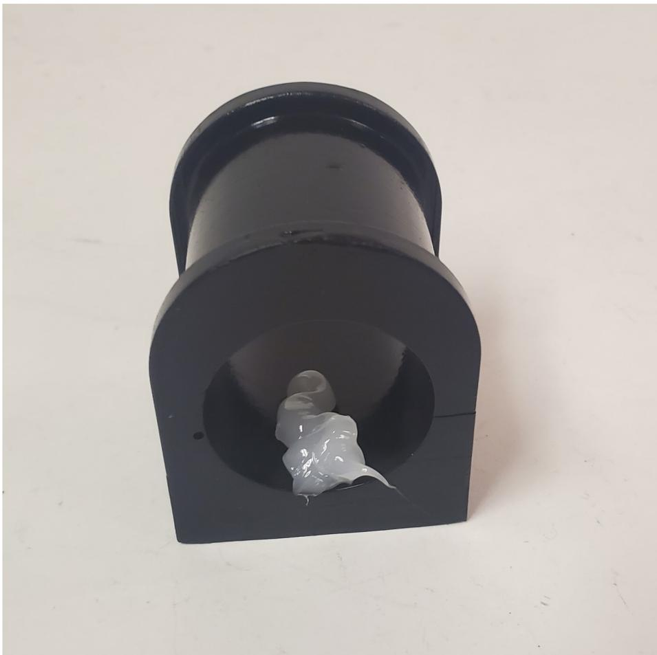
Apply ample amount of lubricant to the inside of each D-Bushing. Spread it evenly throughout the entire inside of the D-Bushing.
