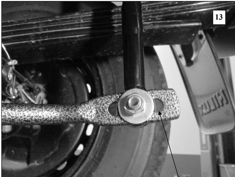
Attach end link to end hole prior to initial use. Center hole is to be used for fitment only and not for initial setting. **After driving vehicle, a firmer setting may be selected if desired.**
