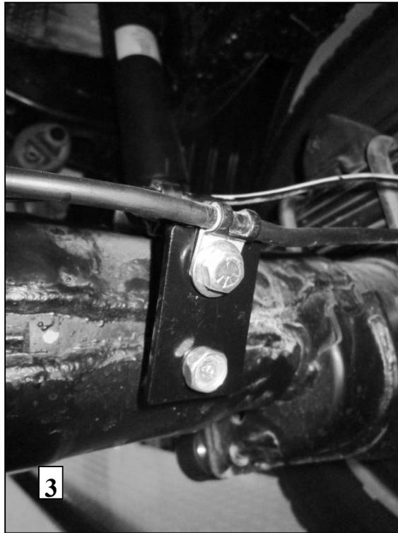
1. Remove bolt attaching driver side brake line to axle tube as shown in photo 2. Flip it over and attach to the tab above using the factory bolt to pull the brake line up.
