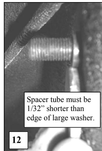
11. Review end link mounting detail on the next page before drilling holes. Note—3/4" spacer will take the place of the thick washer shown in the diagrams. **BEFORE DRILLING ANY HOLES IN THE RAIL—RELOCATE AND PROTECT ANY FUEL OR BRAKE LINES THAT MAY INTERFERE WITH THE DRILL BIT OR SWAY BAR INSTALLATION.**
