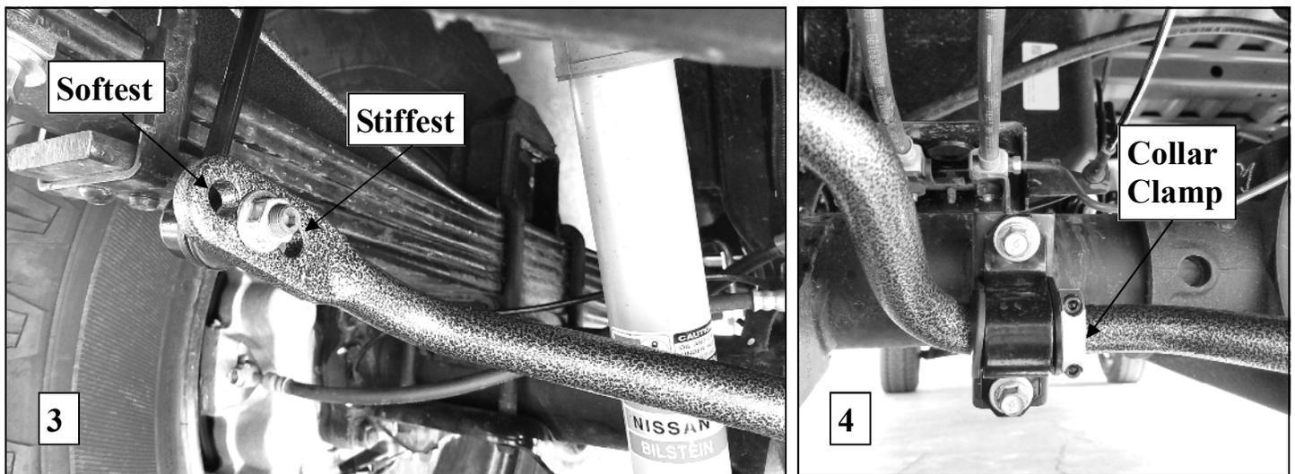
1. Remove the factory installed anti sway bar and the mounting hardware leaving the end link attached to the vehicle. Do not discard the hardware as it will be re-used.
