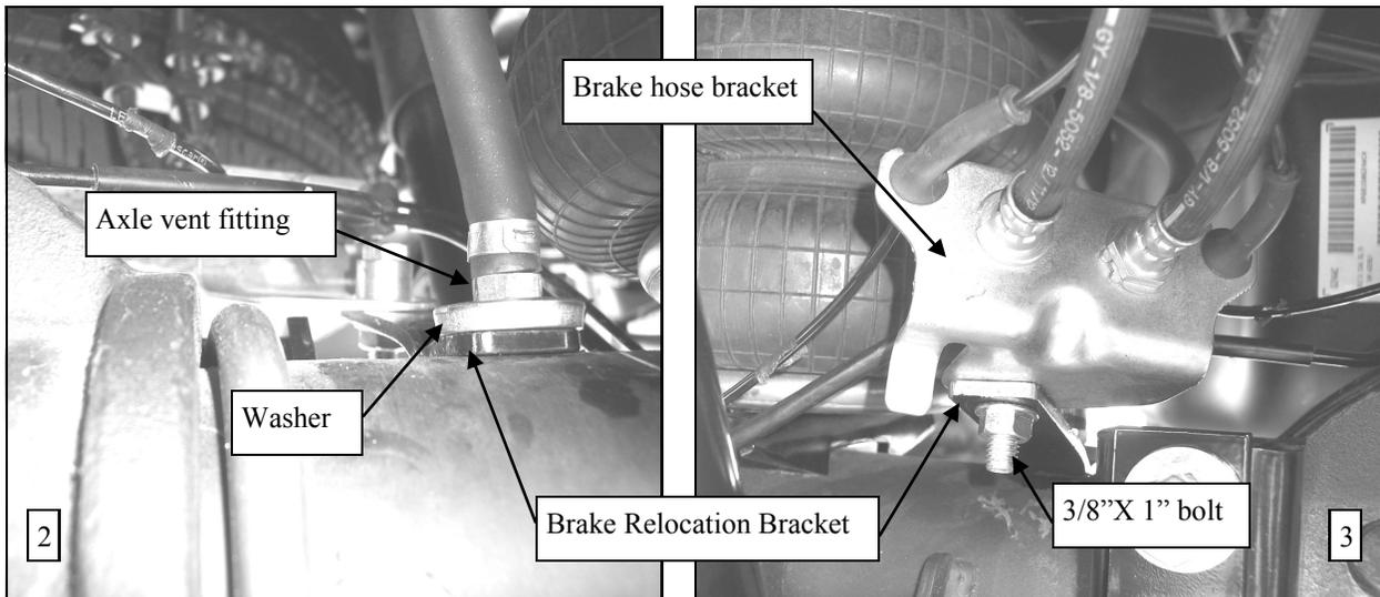
1. Locate threaded axle vent fitting attached to axle and remove threaded fitting to separate the brake hose bracket from the axle.
