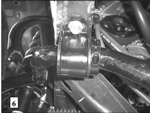
12. After all adjustments have been made, tighten the collar clamp bolts to 5-8 ft-lbs and the other bolts to factory specifications.
