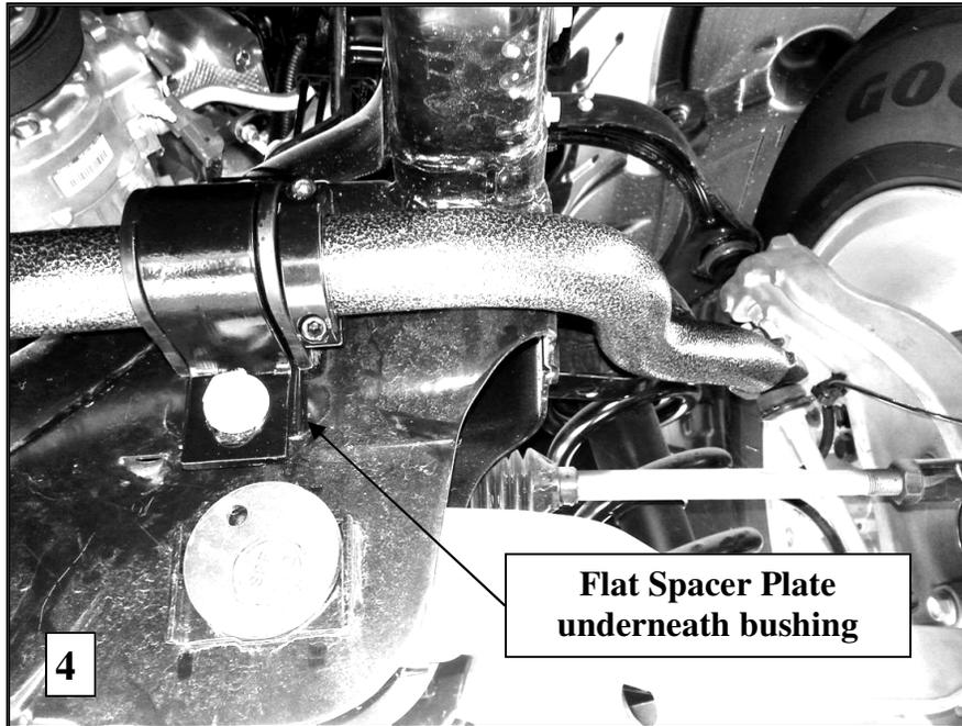
1. Remove the factory installed anti sway bar and the mounting hardware, leaving the end links attached to the control arms. Do not discard the hardware as some of it will be reused.
