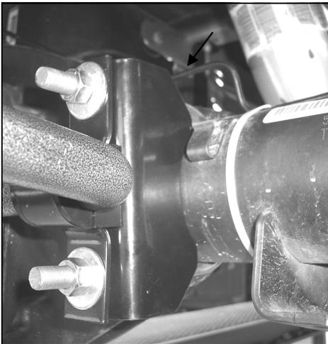
9. Thread jam nut and hex nut on to threads of end link far enough to mount flat washers and bushings to the end of sway bar as shown in photo three (3). Attach sway bar to end link using locknuts provided in kit. **LEAVE LOOSE AT THIS TIME** to allow for adjustment later.
