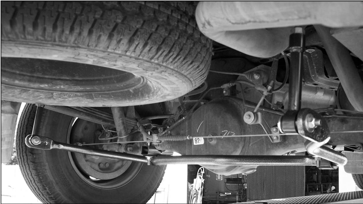
9. With the bar properly aligned, verify that all vehicle components have proper amount of clearance, and that brake lines, wires, cables, and other components will not be pinched or crushed when u-bolts are tightened. Torque U-bolts to 35 ft-lb.
