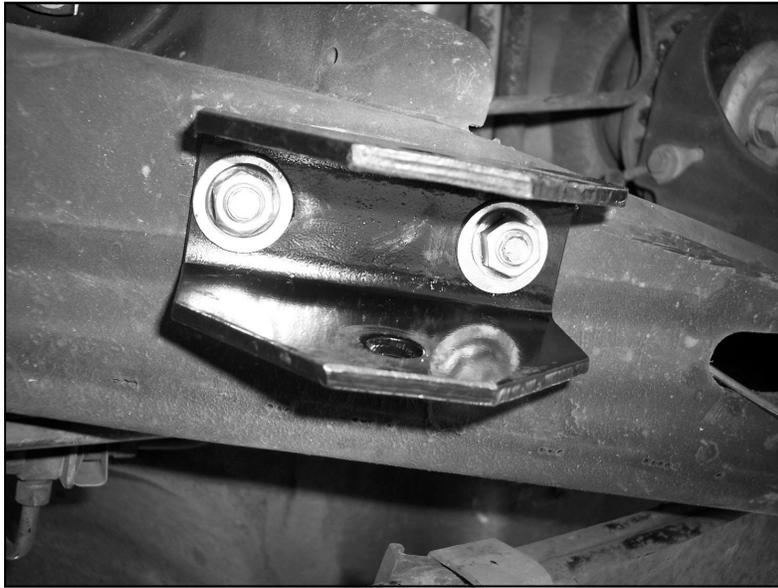
10. Attach frame bracket to rail with 3/8" flange nuts and washers. Torque to 20-25 ft-lb.
