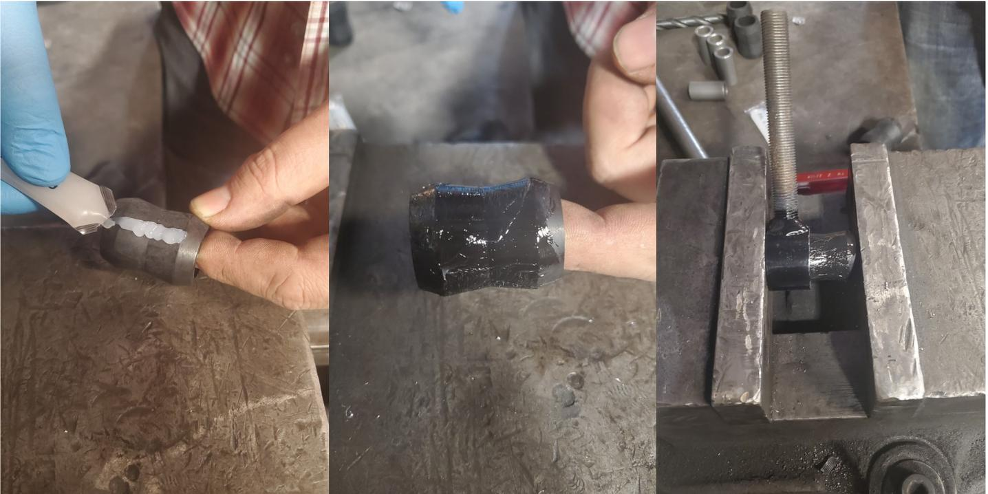
When installing the hour glass end-link bushing, remember to use lube. This will not only aid in ease of the hour glass bushing installation, but also reduce squeaking of the suspension.
