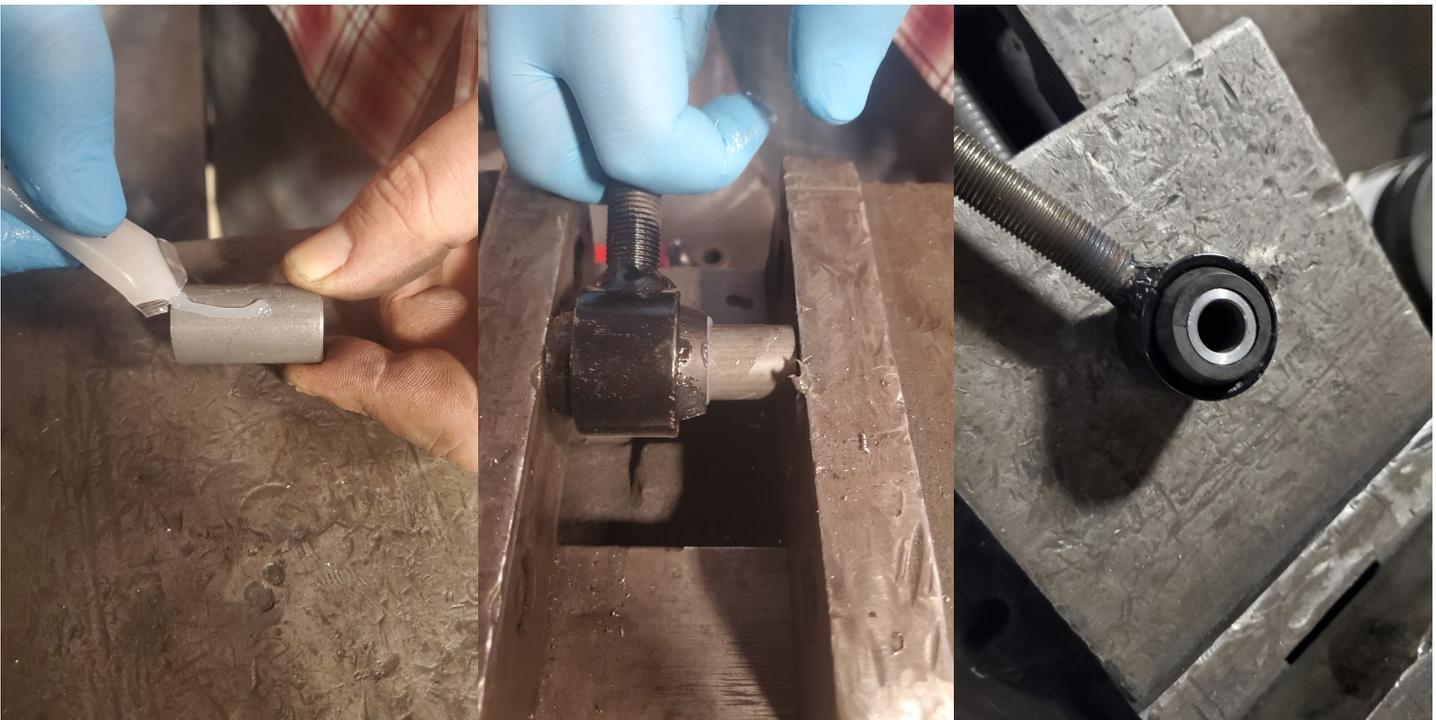
Next, take the bushing sleeve and lube the outside of it. Spread the lube around evenly.
