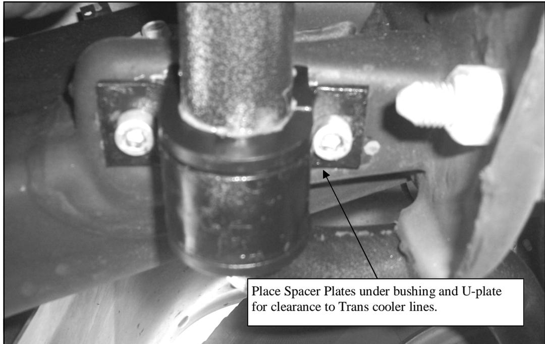
1. Follow 7685 instructions and keep factory mounting hardware attaching U-plate to frame.
