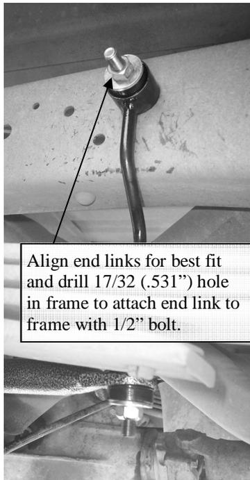
Align end links for best fit and drill 17/32 (.531") hole in frame to attach end link to frame with 1/2" bolt.
