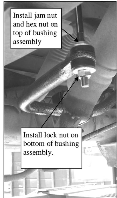
Install jam nut and hex nut on top of bushing assembly
