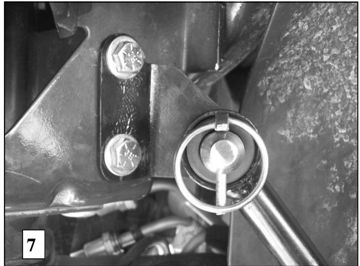
7. Attach the quick disconnect pins to the existing lower end link mounting bracket following Diagram 4 and Photo 2 on the previous page. Use the included longer, 1/2x1-1/2" bolts. Torque bolts to 40 ft-lb. A small Phillips screwdriver can be inserted in to the hole in the end of the pin to keep it from turning while tightening bolt.
