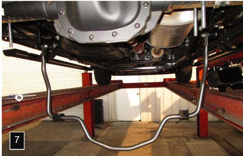
6. Attach end holes of the sway bar to end links using 7/16 x 2-3/4" bolts, washers, and locknuts as shown in photo 7. Leave loose at this time.
