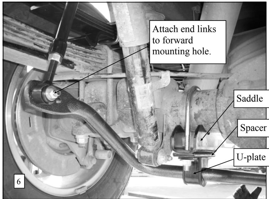
7. Lubricate and install polyurethane D-bushings and U-plates on the sway bar in the locations shown in photos 4&5.
