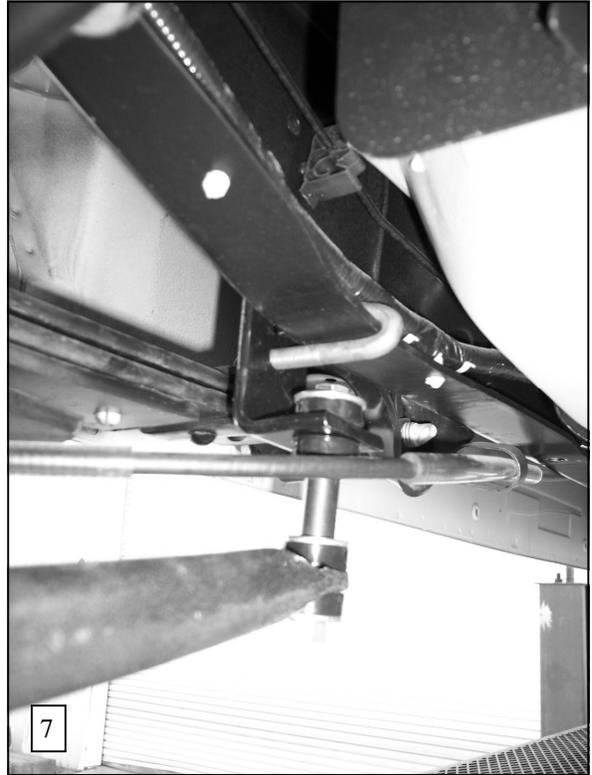
5. Attach angle bracket to frame rail by locating the welded bolt/plate assembly on the inside of frame rail and attaching angle bracket using 1/2" locknut and washer. **Leave loose for adjustment later.**
