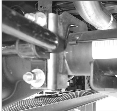
7. Thread jam nut and hex nut on to threads of end link far enough to mount flat washers and bushings to the end of sway bar as shown in photo three (3). Attach sway bar to end link using locknuts provided in kit. **LEAVE LOOSE AT THIS TIME** to allow for adjustment later.
