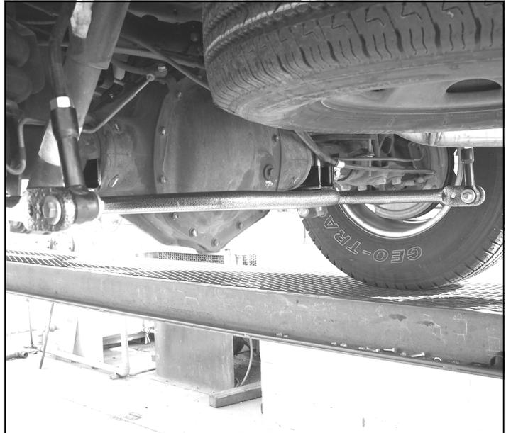
12. Center sway bar on axle and tighten axle U-bolts to 60 ft-lb. Double nut axle u-bolts after torquing to spec.
