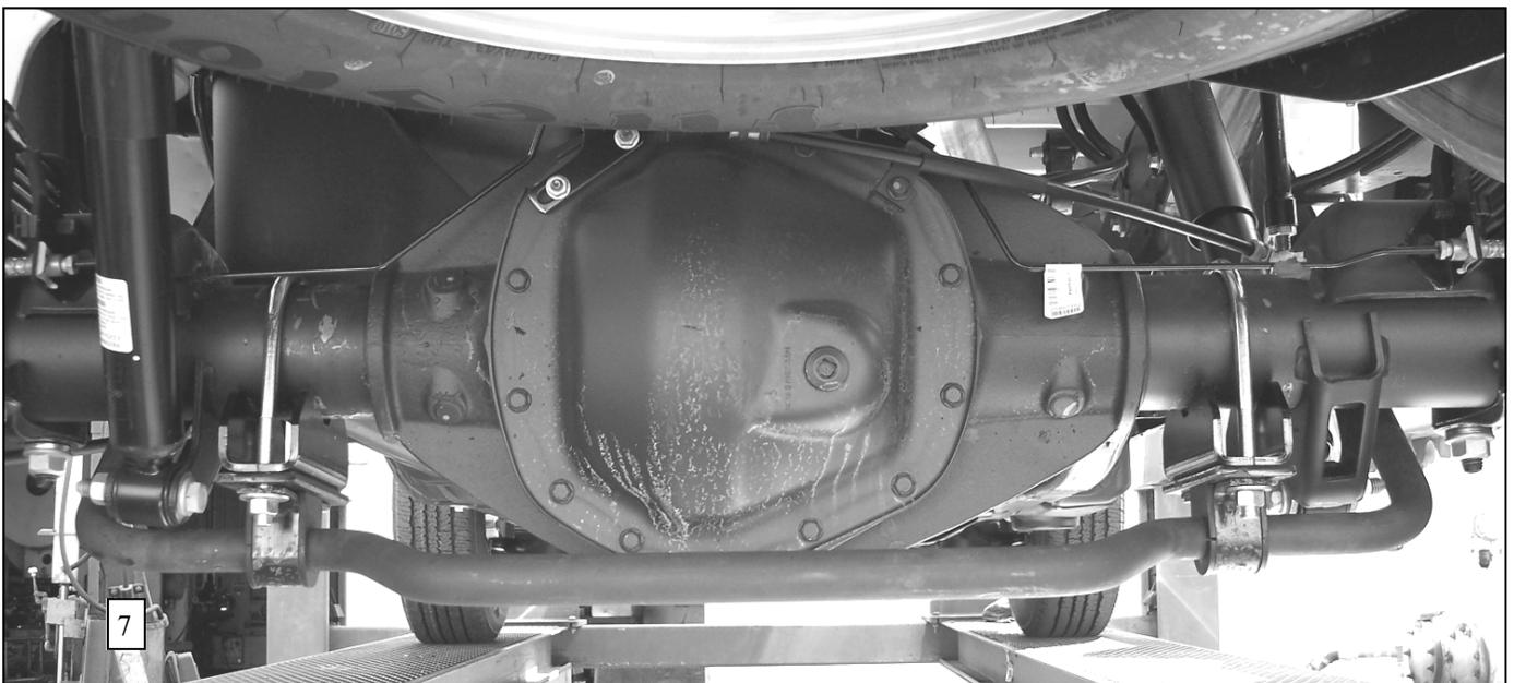
12. After all adjustments have been made, tighten end link mounting bolts to 35-40 ft-lb and 9/16" adjustment nut on end links to 70 ft-lb.
