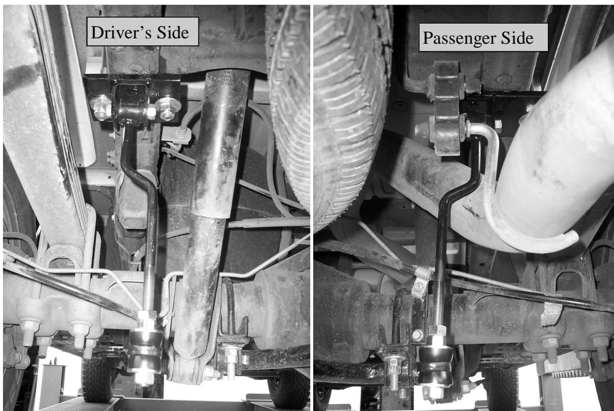
5. Locate existing spare tire crossmember on vehicle frame. Place square U-bolt over the frame rail in front of the crossmember with legs of the U-bolt pointing downward.
