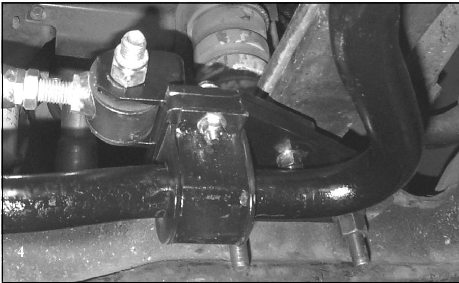
6. With frame bracket & axle plates installed, attach the anti-swaybar on the bottom of the axle plates using the D-bushing & U-plates. (See picture 3). Orient the hump of the swaybar down & the arms forward towards the front of the coach. Leave bolts loose enough for adjustment later. Connect the swaybar to the endlink using hardware provided. Center the swaybar in the U-plate so that the bar lines up with the endlinks. The endlinks should be straight in line with the swaybar at this time.
