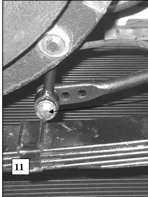
Attach end link to outer hole as shown before driving. DO NOT use inner holes until first driving vehicle with end link in outer position.
