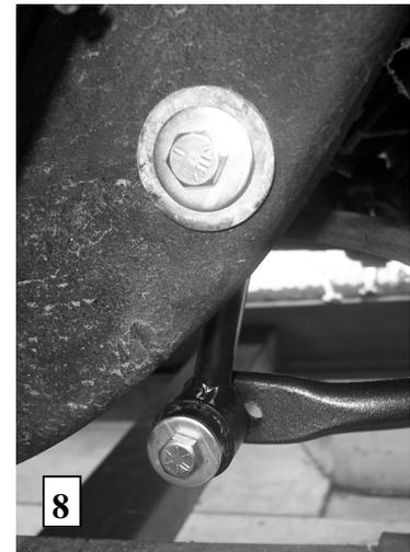
20. **Bounce the vehicle checking for clearance on all under carriage components: fuel tank, shocks, differential, brake and fuel lines, etc.** Test drive the vehicle and recheck all clearances and the installation alignment. Adjust as needed. Re-check your installation after one week of driving and periodically on a regular basis.
