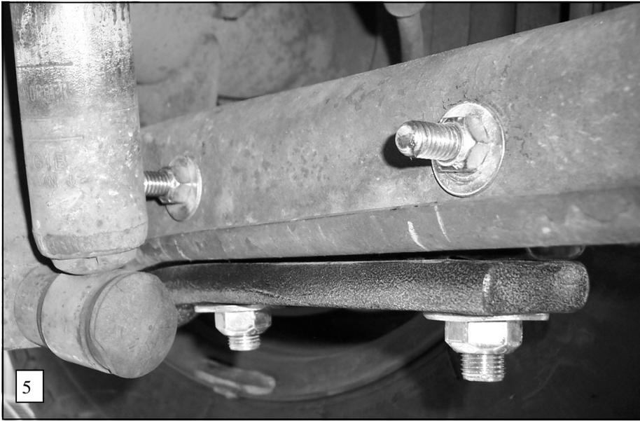
4. Insert 3/8 x 2-1/4" bolts into holes in control arm and fasten assembly with washers and locknuts as shown in photo (5).
