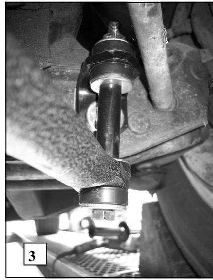
1. If equipped, remove the factory installed anti sway bar and the mounting hardware.
