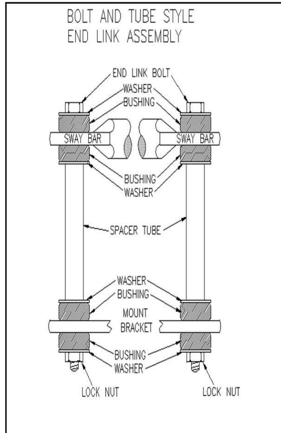
8. Assemble end links as shown in photos 3&7 and diagram. Tighten end link nuts until bushings start to bulge slightly.
