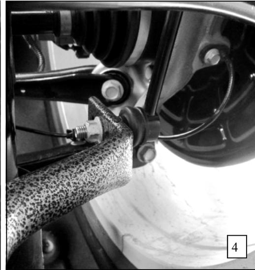
10. Attach the factory end links to the center hole on the sway bar using the factory nut as shown in Photo 4. Torque to factory specs.
