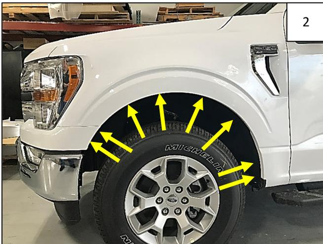
Using a 7mm socket, remove 8 factory screws from wheel well. Retain all screws for reinstallation. NOTE: Some models may not have screws in some locations; we have provided #8 Truss-Head Screws in this case.
