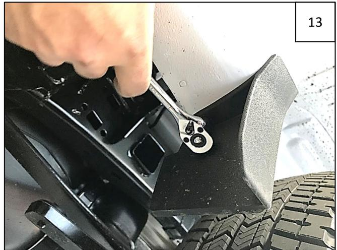
Remove a 3<sup>rd</sup> screw from underside of lower front of wheel well.
