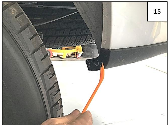
Using a pry tool, remove outermost factory plastic fastener from lower rear of wheel well (inner fastener remains). Discard. Leave inner plastic fastener installed.
